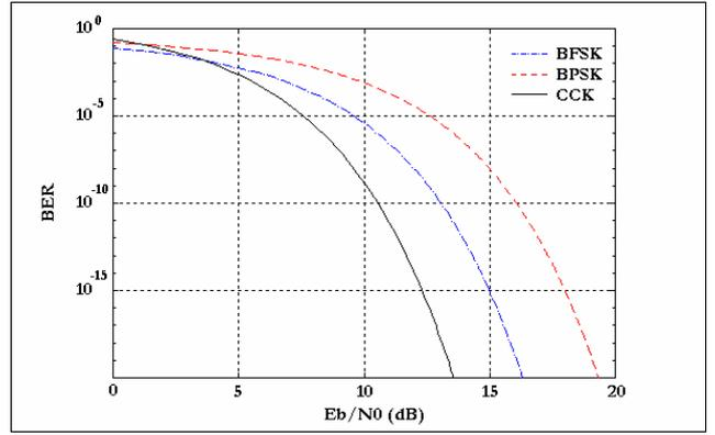
Fig. 2. SNR and BER for some digital modulation schemes
