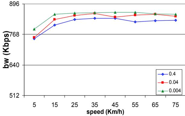
Fig. 6. Allocated bandwidth to MIP services for different outage probability  $p_0$  and speed values.
