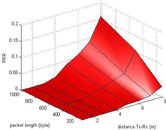
Fig. 4. PER vs. packet length and distance for rate 110Mbps in LOS scenario with variance noise  $10^{-2}$ .
