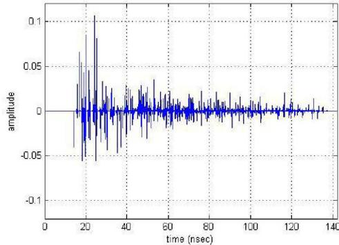
Fig.1. Impulse Response for NLOS scenario with Tx-Rx distance =5m.
