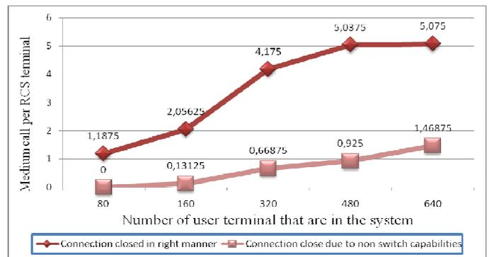
Fig. 6 Right closed call vs. closed call due to no SDR Terminal capabilities.
