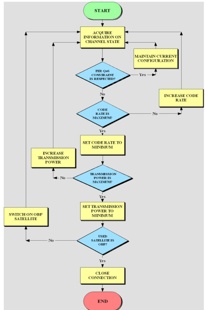
Fig. 3 SPV Algorithm flowchart.
