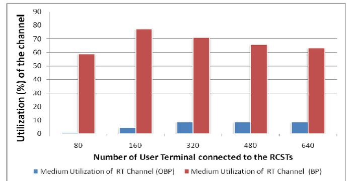
Fig. 7 Utilization of Satellites Return Channel.
