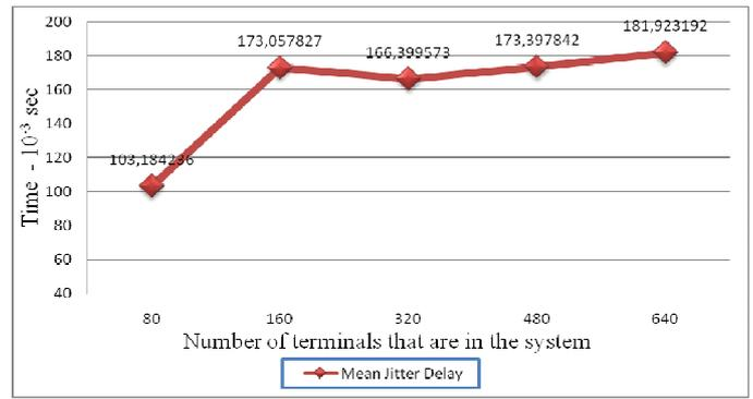
Fig. 8 Average Jitter vs. user terminals augment.
