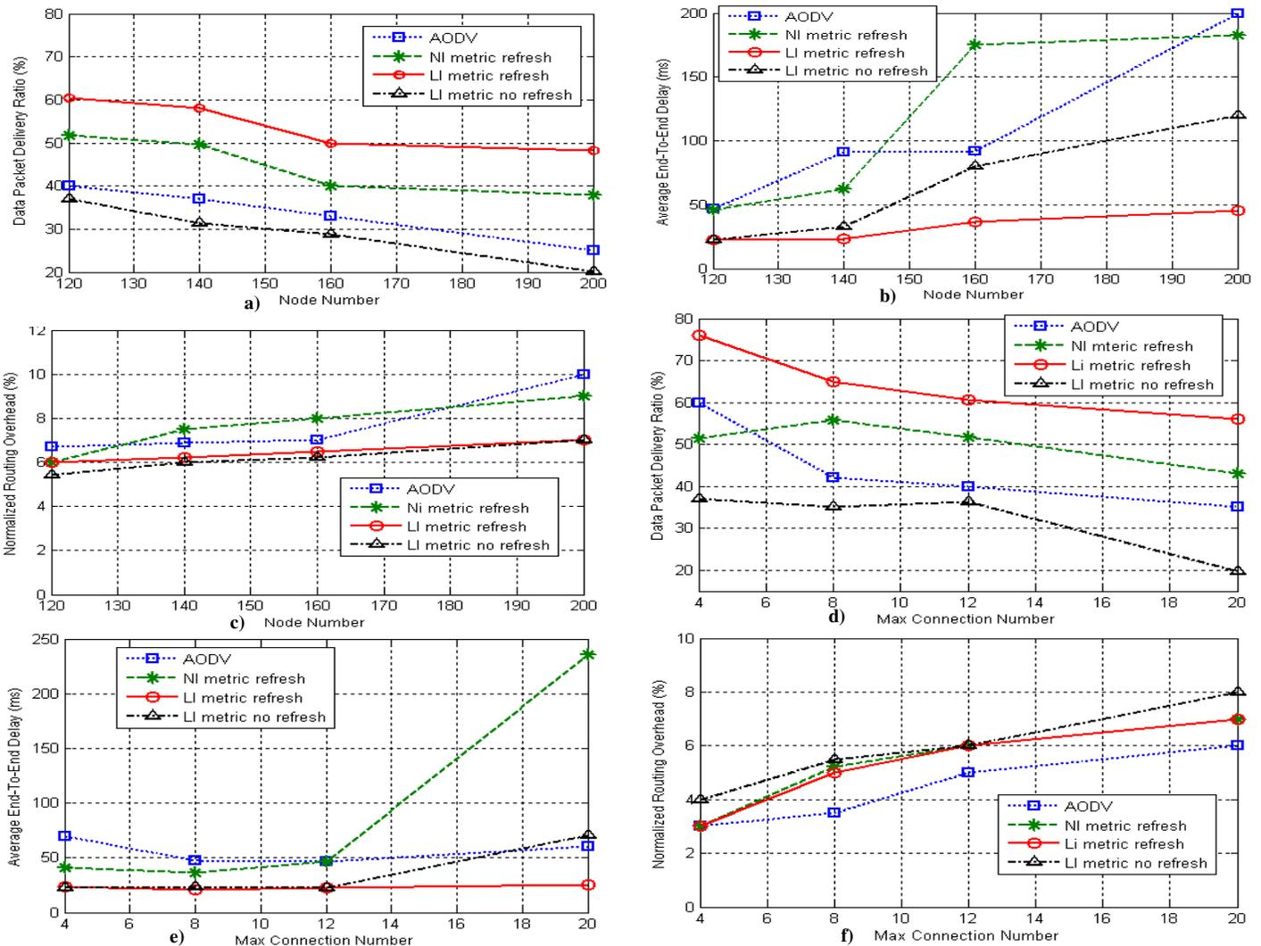
Figure 4. a) PDR vs. node number in presence of 12 maximum concurrent connections. b) AED vs. node number in presence of 12 maximum concurrent connections. c) NRO vs. node number in presence of 12 maximum concurrent connections. d) PDR vs. concurrent connection maximum number with 120 nodes. e) AED vs. concurrent connection maximum number with 120 nodes. f) NRO vs. concurrent connection maximum number with 120 nodes.
