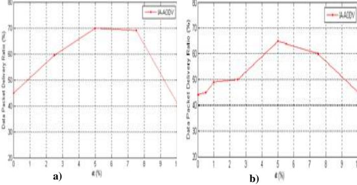
Figure 3. a) PDR vs.  $\alpha$ , 4 maximum concurrent connections, 120 nodes. b) PDR vs.  $\alpha$ , 8 maximum concurrent connections, 140 nodes.
