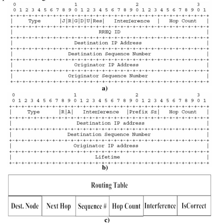
Figure 1. a) RREQ packet structure. b) RREP packet structure. c) Routing table entry.
