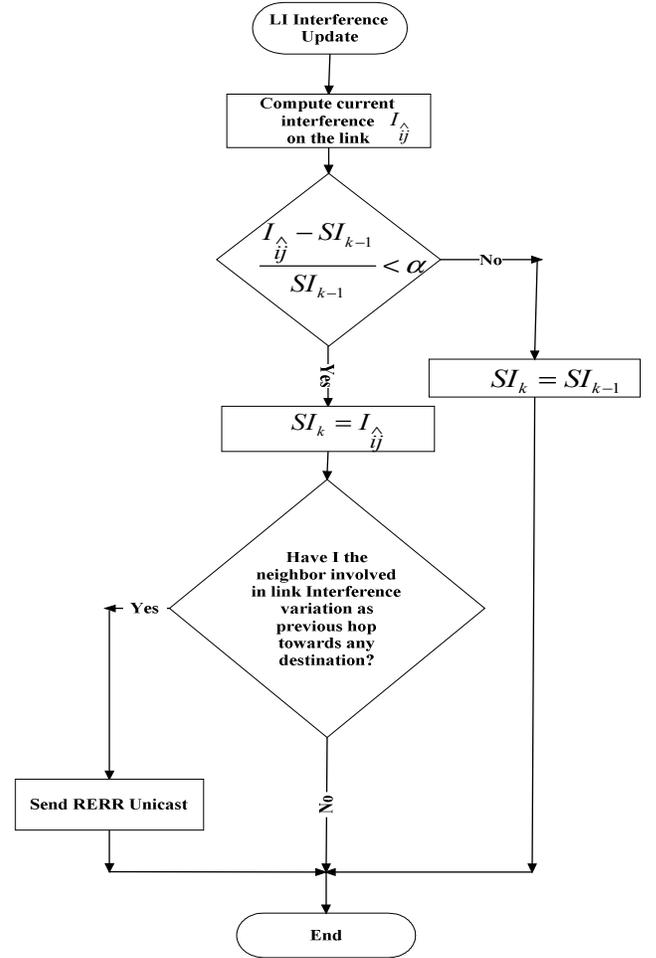
Figure 2. Interference Control on a generic link for the LI metric.
