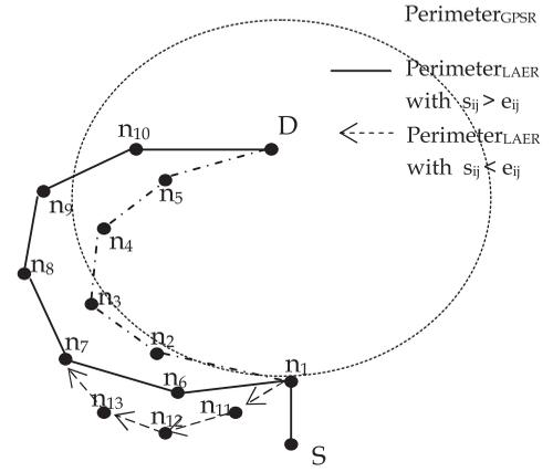
Fig. 2. Perimeter forwarding in *GPSR* and *LAER* protocols.
