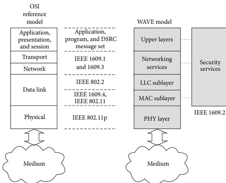
FIGURE 2: WAVE layering compared to ISO reference model.
