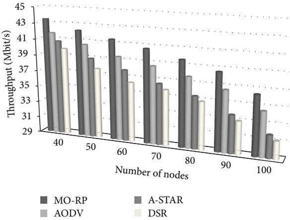
FIGURE 11: Average aggregated throughput versus the number of mobile nodes.
