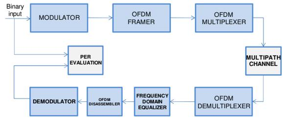
Fig.3: MATLAB/Simulink conceptual scheme of the IEEE802.11p.
