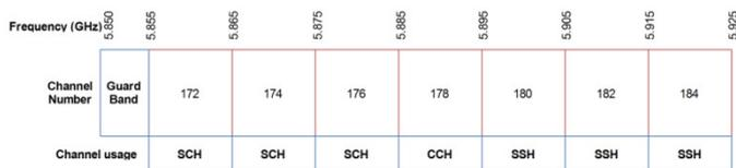
Fig. 1: Frequency spectrum subdivision for DSRC.
